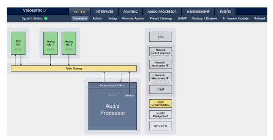
The graphical overview shows the main building blocks of the device including the options installed, in this example the microphone interface is placed into the INTERFACE 2 (see rear view) and a MADI I/O module is placed into INTERFACE 1 slot.
