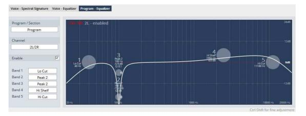
The parametric EQ for the program path offers 5 bands in a similar way as for the voice EQ. Pls. refer to the explanation above. **Program / Selection** has no option because this is for the "**Program**" path. **Channel** depends on the Link mode of the program path. If linked **2L/2R** appears in that field.
