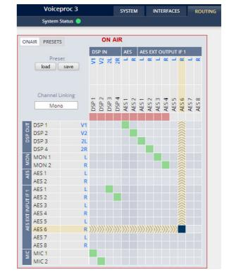
Each functional block of the device has a source label and a destination label. Additional **blue** signal labels give an indication of the type of signal that is expected or issued by the respective function block or I/O interface (e.g. L/R for AES or 2L/2R for DSP 3/4 and so forth).
