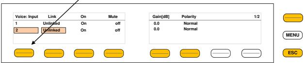
The examples above demonstrates the general way how to setup parameters of the **AUDIO PROCESSOR** of the **D\*AP4 VAP**:
