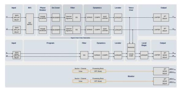
Above you see the various function blocks of the audio processor rendered by the **DSP** engine. Each function block has its representation in the GUI by individual tab sheets. You may simply click on the respective graphical area as an alternative way to navigate through the GUI.
