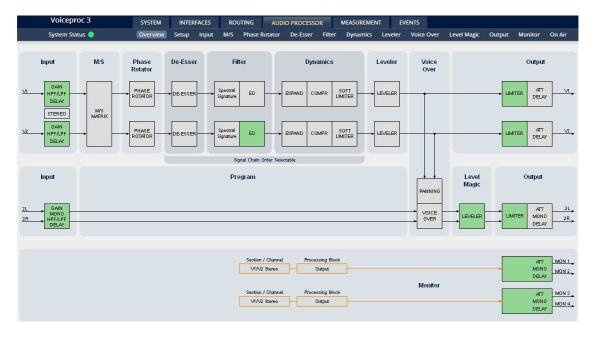
The processing blocks in use, which may be activated from their individual setup panes, will be indicated in green. I.e. blocks shown in grey are not activated by the user.
