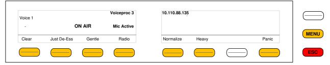
Now you may fire the pre-set actions (see EVENTS > Actions > Event Actions) via the hotkeys. You may configure these buttons via: EVENTS > Triggers > Remote Hotkeys **and** > Trigger Equations. Operating - menu structure of the X\*AP RM1 remote panel - operating displays
