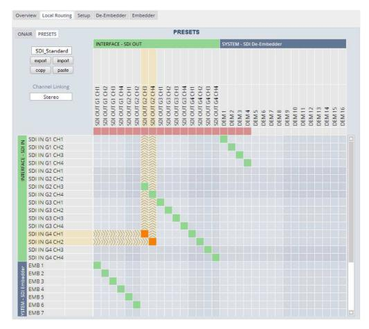
You must use the scroll bar to navigate through the matrix. In the upper left corner you can select between the **ONAIR** and the **PRESETS** view of the matrix. On the **ON AIR** page you will also see the device signal labels (see ROUTING section further below for details).
