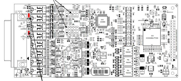
The two jumpers above may lift the shield pins for CH1/1 and CH3/4 from analog ground to HF coupling.
