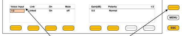
Here you are at the input **•** section of the voice channel. The **<Shift**> **•** button again toggles between two pages and gains access to the remaining parameters.
