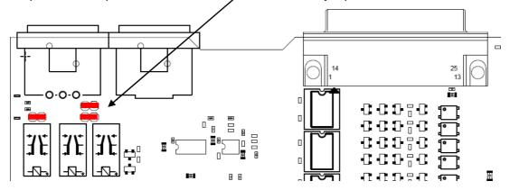
You must remove the jumpers to de-activate the AES I/O relay power fail circuit.
